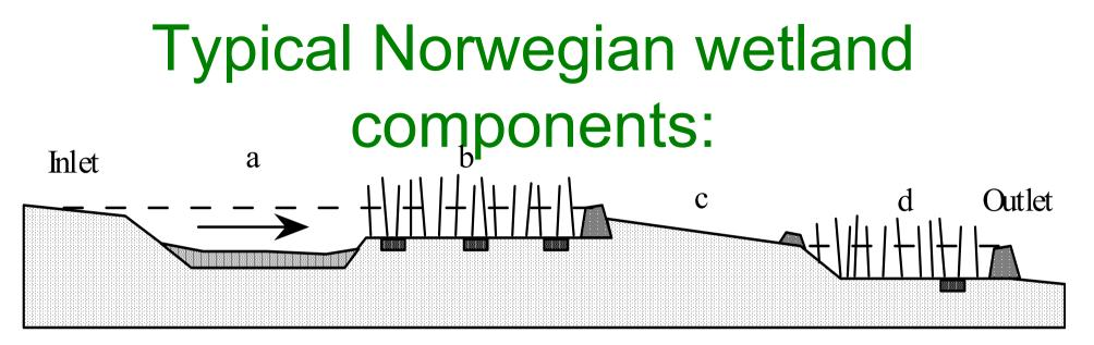
Sedimentation pond (1-2 m) Vegetation filters (0.3-0.5 m) Overflow zones (0-0.1 m) Vegetation filter
